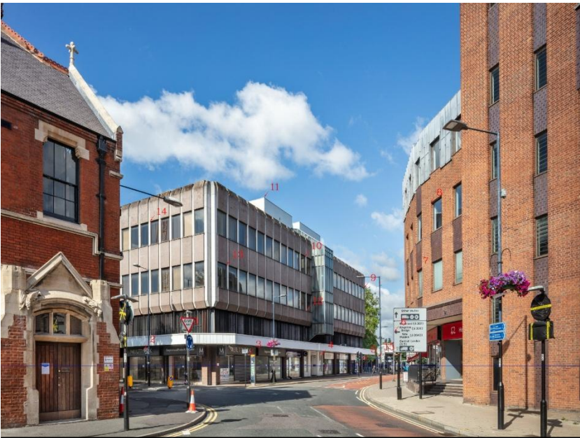
Red markers placed at surveyed OSGB36 coordinates in the 3D model. Each must align precisely with its counterpart in the photograph before rendering is approved.
