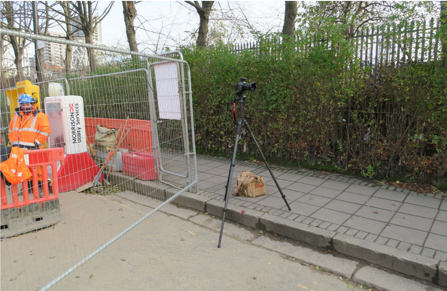
Camera and tripod in position over the surveyed mark
